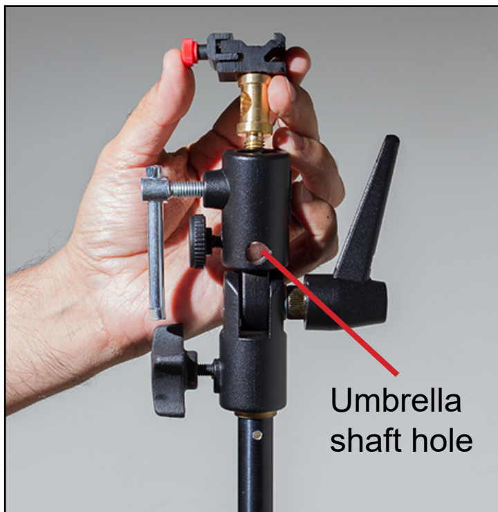
Figure 2.3. Cold shoe and stud being attached to an umbrella adapter.
