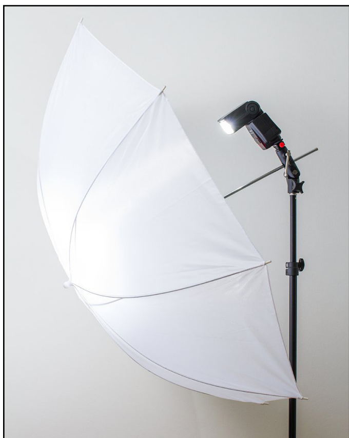
Figure 2.6. Umbrella shown in the shoot-through orientation. Rather than have the umbrella bounce/reflect light from the flash onto the subject, the top of the umbrella is directed toward the subject providing a kind of “open softbox” effect.
