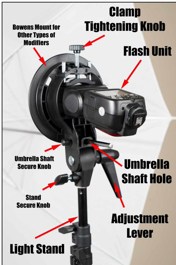
Figure 4.3. Close-up view of light stand setup. This flash has a built-in radio receiver so an external radio receiver is not necessary.
