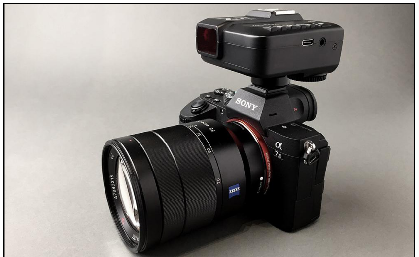
Figure 2.8. Third-party radio flash trigger compatible with my camera's brand of TTL. This transmits signals to compatible remote flash units in either manual or TTL modes.
