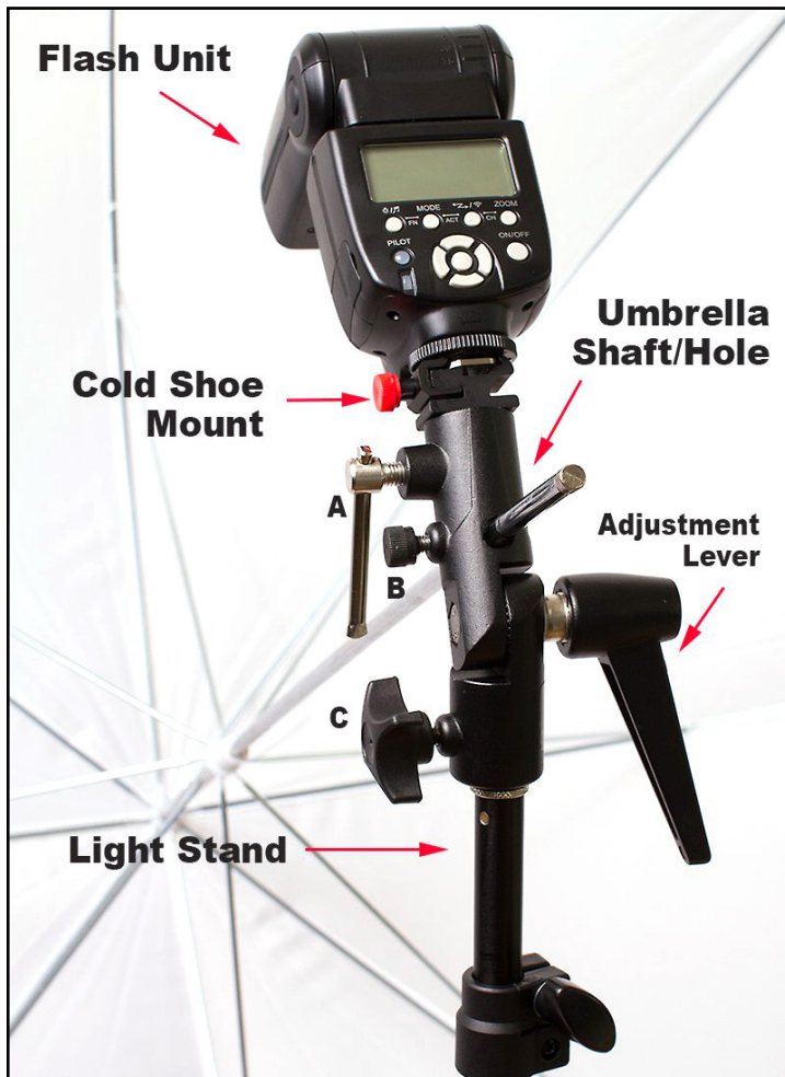
Figure 4.1. Close-up view of light stand setup. This flash has a built-in radio receiver so an external radio receiver is not necessary.
