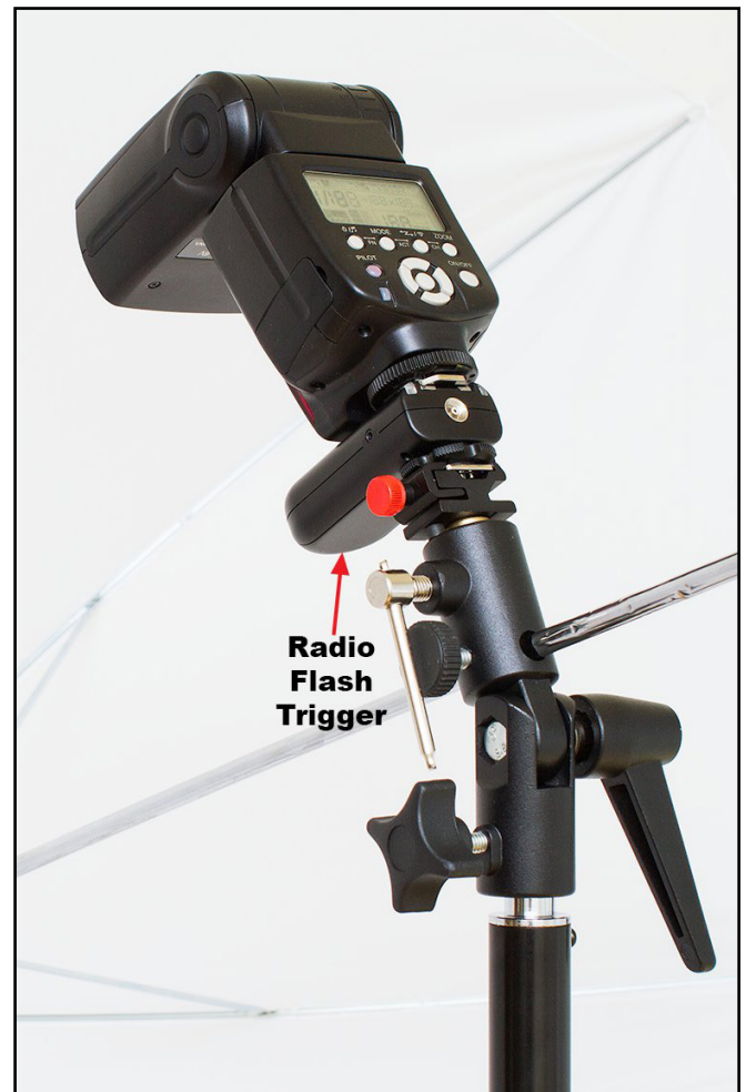
Figure 4.2. Light stand setup showing the flash mounted to a flash trigger receiving unit.
